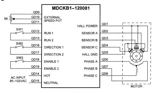
Note: The MDCKB1-120081 driver is not line isolated. Use only mechanical switches for the control inputs. The terminals of motor connector contains high voltage. Do not probe any part of the driver with power on, this could damage the drive or result in body injury.
